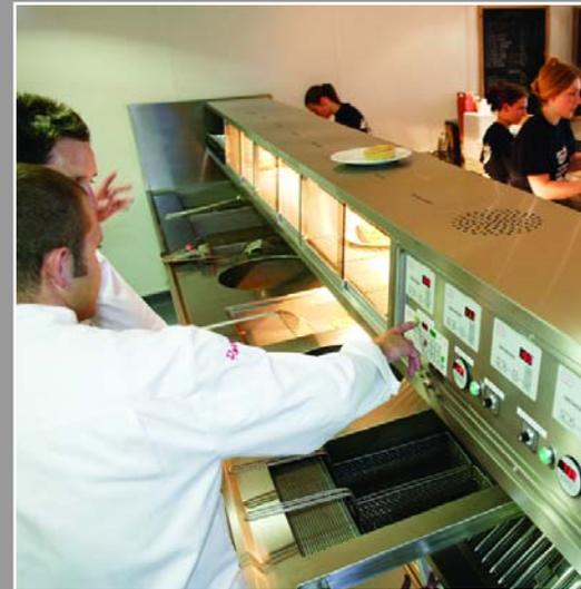
A Flotronic controller has three different temperature programmes and twelve different timers - with load compensation available for each pan.
